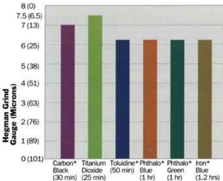
\*Note: The final grind capability depends on formulation. Some of these hard pigments are difficult to reach a 1-4 Hegman on a rotor/stator mill.
